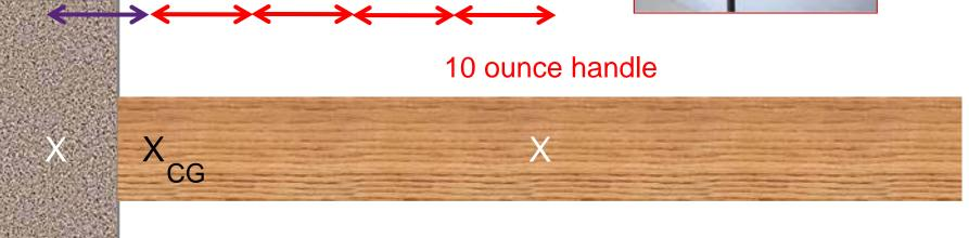
For example, if the head is 4 times heavier than the handle then CG is 4 times closer to the center of the head than to the center of the handle.
